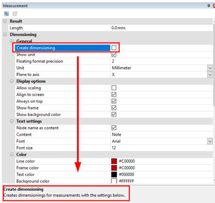
A screenshot of the 'Measurement' dialog box. The 'General' section is expanded, showing settings like 'Show unit' (checked), 'Floating format precision' (set to 2), 'Unit' (set to 'Millimeter'), and 'Plane to axis' (set to 'X'). A red box highlights the 'Create dimensioning' button at the top of the list. A red arrow points from this button down to a red box around the explanatory text at the bottom of the dialog: 'Creates dimensionings for measurements with the settings below.'. |
